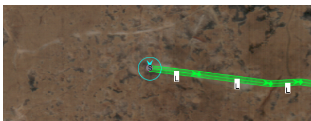
Figure 12: Typical visualization of the connector a treeline is member of. The connector is depicted with a circle around the base node of the treeline and an arrow head pointing at this base node.
